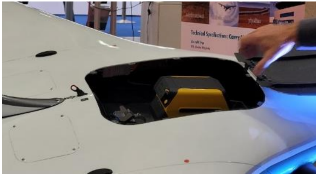
Fig 1. Installed Yellowscan Explorer
